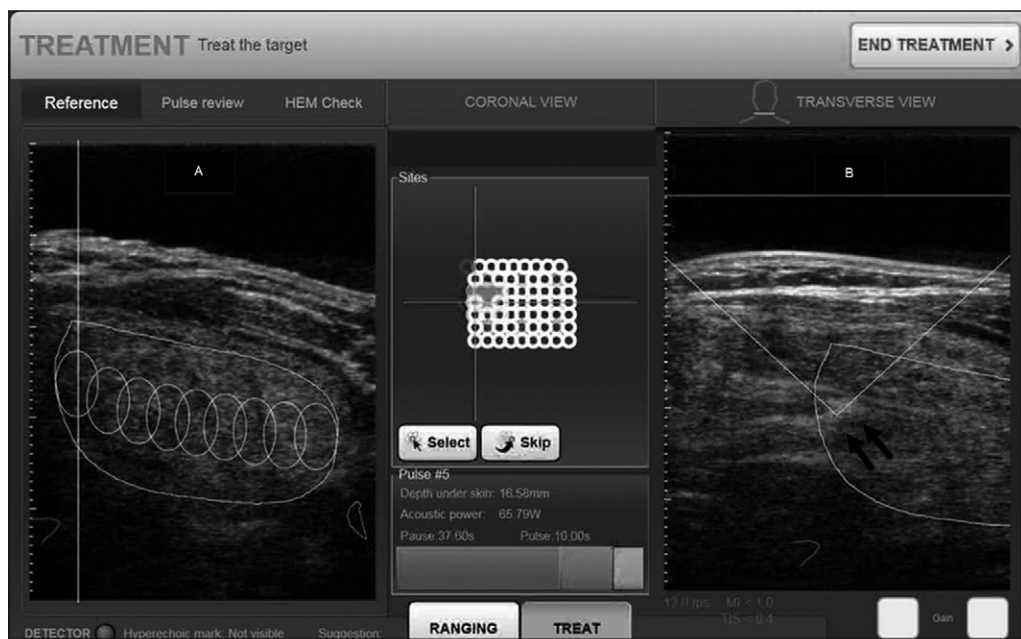
Figure 1: (a) Touch-screen interface of HIFU machine. Central panel shows top view reconstruction of nodule, which is made of multiple white circles. Empty circles represent unablated subunits and filled circles represent ablated subunits. Image A is the planned image, and image B is the actual real-time image during treatment. Hyperechoic marks (a sign of tissue necrosis) are indicated with two black arrows on image B. (b) US images were obtained before treatment, immediately after, and at 3, 6, and 12 months after treatment.
