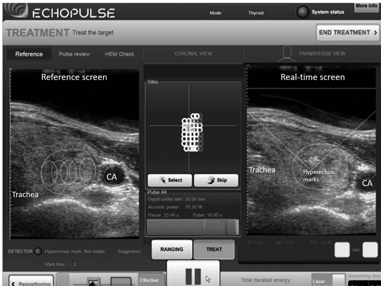
Figure 1. Treatment screen. The central panel shows the top view reconstruction of the nodule which is made up of multiple white cycles. The empty circles represent the un-ablated subunits while the filled circles represent the ablated subunits.
